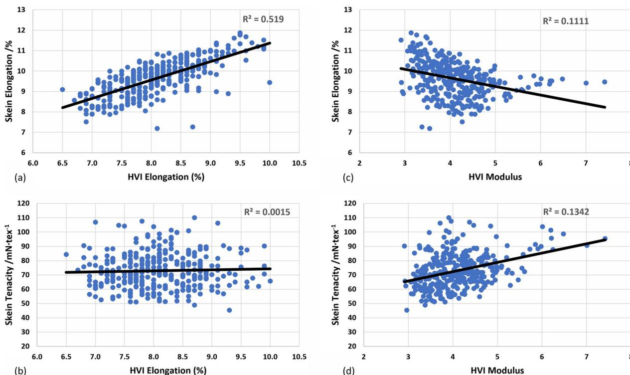
**Fig. 2** a HVI Elongation (%) vs Skein Elongation (%). b HVI Elongation (%) vs Skein Tenacity (mN/tex). c HVI Modulus vs Skein Elongation (%). d HVI Modulus vs Skein Tenacity (mN/tex)
