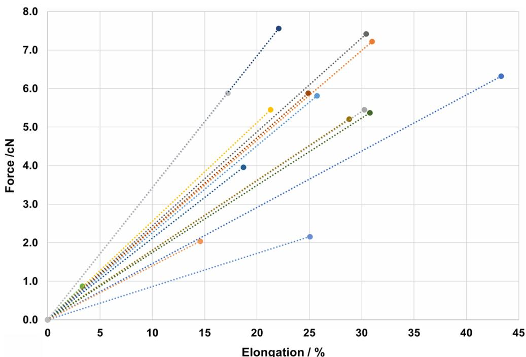
**Fig. 1** The force elongation curve of 15 randomly selected fibers from DPL 1612B2XF cotton grown in 2018
